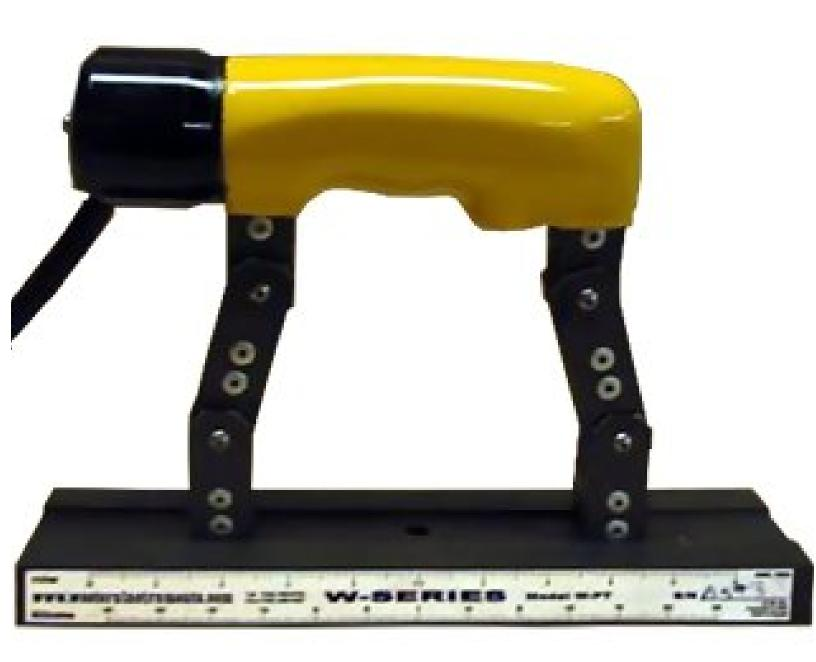
The WC-42 is an AC Yoke which induces a magnetic field into the ferrous material being tested. The unit should be used within the parameters as set out in the specifications within this guide. This Manual also applies to similar Low Voltage Models such as the WC-48.
